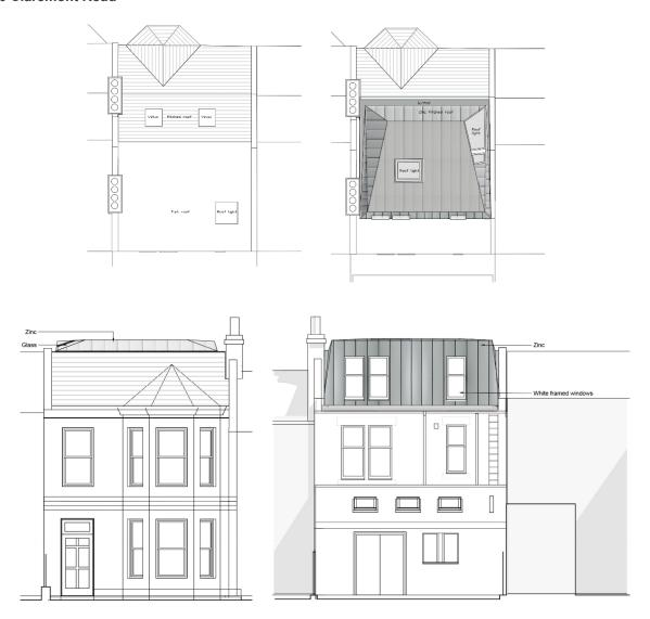
Figure 22 – Existing roof plan (top left), proposed roof plan (top right) and elevation proposals (below plans) for 20 Claremont Road
